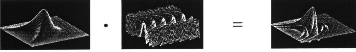
Figure 3: A banana wavelet (real part) is the product of a curved Gaussian G^{\vec{b}}(x, y) and a curved wave function F^{\vec{b}}(x, y) (only the real part of the kernel is shown).
